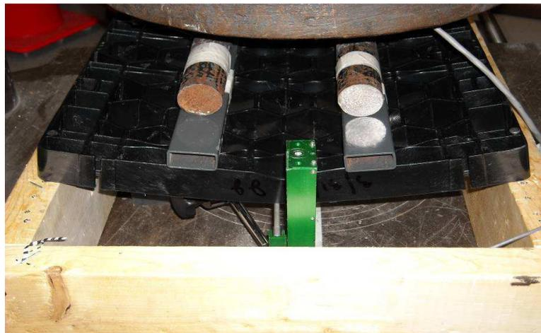
**Figure 3: Silca Grate under load at 1.5” deflection**
